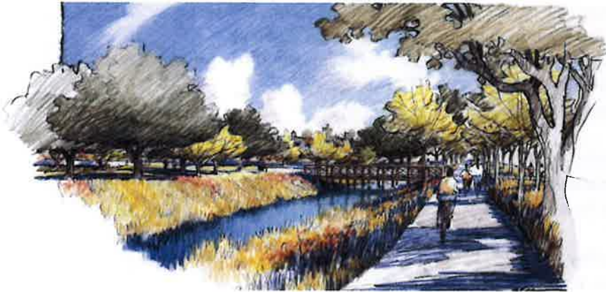
Figure 5.2 illustrates a 150-foot section of the Laguna South Grand Parkway. A 10-foot Class I bike trail is proposed on one side of the channel.
